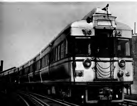
First all-electric PCC rapid transit cars for Chicago underwent their trial runs in 1948. They represent the first of a series of steps leading to the high-performance cars of 1968.
